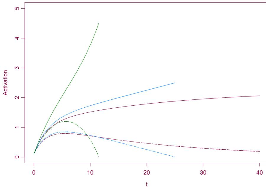
Figure 3. Solid lines indicate the unit with larger input, dashed lines the unit with the smaller input, red lines indicate  $N = 0$ , blue  $N = 1$ , and green  $N = 50$ . Plots are terminated at quenching, except for  $N = 0$ , where quenching does not occur in a finite time.
